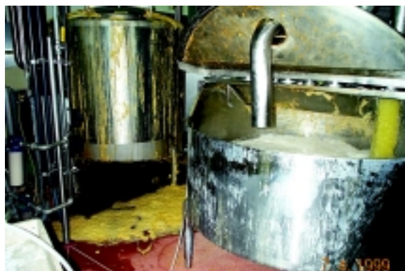
This spill in a dairy products operation resulted from a non-automated High Temperature Short Time cleaning process that produced periodic losses of water and energy due to lack of consistent control regulation.
