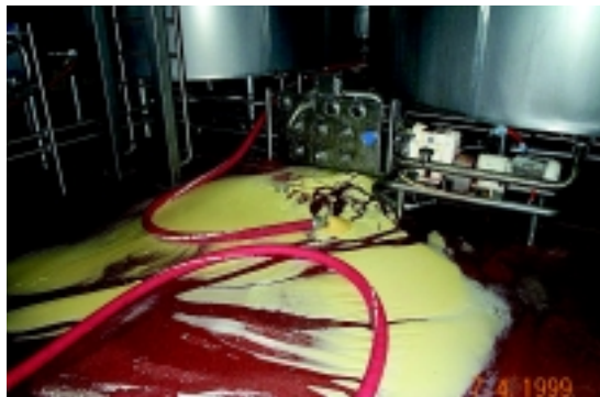
This food product loss and BOD pollution resulted from a bad connection between vats in a whey crystallisation process. Improved training for plant personnel was one remedial approach applied in this case.
